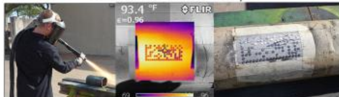
Stenciled HVOF direct to Metal part
