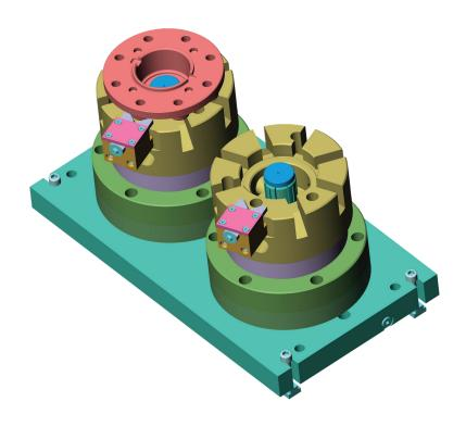
The workpiece is for the automotive industry. The collet grips on the ID of the part and radially locates externally on a cast boss.
