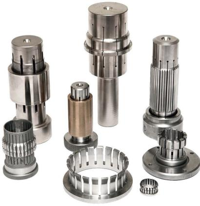
Designed for inspection applications the Push-On Arbor is an economical, durable, and accurate chucking mechanism. The simplicity of its construction provides a greater measure of accuracy at a lower cost. The piece part is simply pushed onto the arbor and gripped by its own inherent forces. There are no actuating components and therefore not subject to influences from cylinder or wrench tightening forces.
