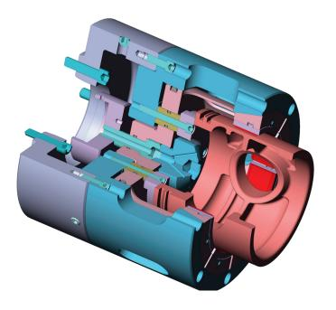
The workpiece is a piston for large heavy duty trucks. Gripping on the OD of the workpiece. The collet has inserts that can be changed for various piston OD's coolant is introduced thru the center to help flush out chips.
