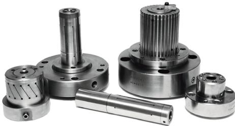
Unlike most hydraulic arbors, our unique adjusting screw feature gives the user the ability to easily re-charge the system, saving critical down time. Standard Tolerances of .0002" T.I.R. Completely repairable if damaged or worn. Can be actuated manually using machine drawbar, and/or external hydraulic source.
